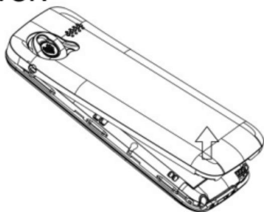
2. Insert 1 or 2 SIM cards (also memory card if you have it). Position for SIM cards is marked by SIM1 and SIM2. Place the
