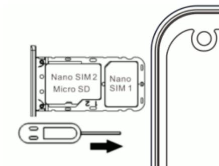
Insert one or two Nano SIM cards in the free slots. You can also insert one Nano SIM and a Micro SD memory card. When using a Micro SD card, only one Nano SIM card can be inserted.
